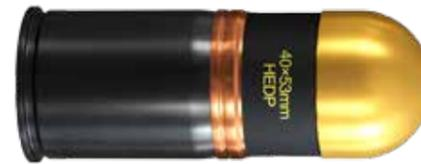
High explosive dual purpose operational cartridge provides simultaneously a lethal blast and fragment radius of 5 meters and armor penetration greater than 50 mm RHA. Suitable for use in Mk19 Mod 3, H&K GMG and other Automatic Grenade Launchers. It may be offered linked with the HE version, in different configurations.
